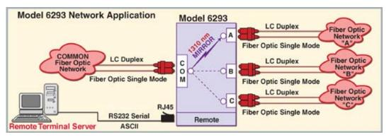
Block Diagram 6: Example of a fiber optic switch with a Remote port which can be used to lockout the front-panel pushbuttons with ASCII commands.
