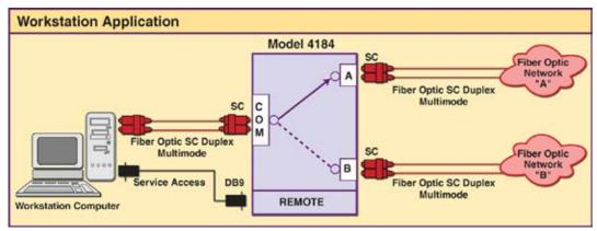
Block Diagram 8a: QuickSwitch® 4184 block diagram illlustrates a Fiber Optic SC Duplex Switch for a workstation application showing fiber optic link backup.
