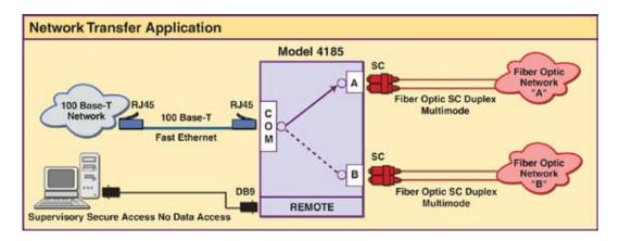
Block Diagram 7: QuickSwitch® 4185 is an example of a password protected Supervisory Remote. Access can be obtained with the proper authentication.
