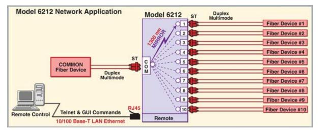
Block Diagram 2: Example of a 10-Position switch.
