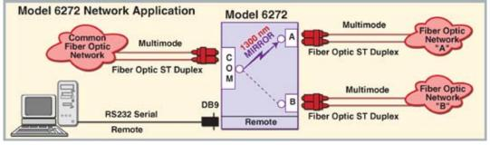
Block Diagram 10: *QuickSwitch*® 6272 ST Duplex Fiber Optic Mirror A/B Switch with Remote Serial Control is an ideal backup switch for high speed requirements.
