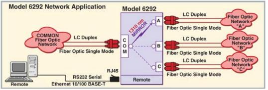
Block Diagram 12: QuickSwitch® 6292 LC Single Mode Fiber Optic Mirror A/B/C Switch with 10/100 Base-T LAN TELNET Access Remote is an IP addressable switch.
