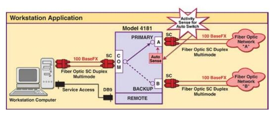
Block Diagram 9b: *QuickSwitch*® 4181 block diagram illustrates a Network Transfer application with a "FAST ETHERNET".
