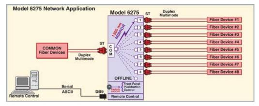
Block Diagram 5: Example of a fiber optic switch with an internal Off-Line position and a keylock to lock out the front panels pushbutton controls.
