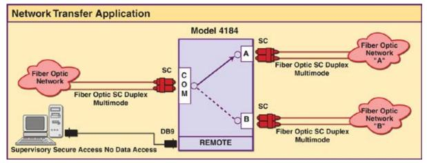
Block Diagram 1: Example of an A/B switch.
