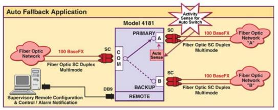
Block Diagram 9a: *QuickSwitch*® 4181 block diagram illustrates a Fiber Optic SC Duplex Switch for a workstation application showing Automatic Fallback based on SD.
