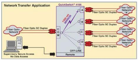
Block Diagram 4: Example of a fiber optic switch with an external Off-Line position with switch position memory.
