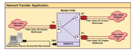
Block Diagram 8b: QuickSwitch® 4184 block diagram illustrates a Network Transfer application with an RS232 Serial security enhanced Supervisory Remote Port.
