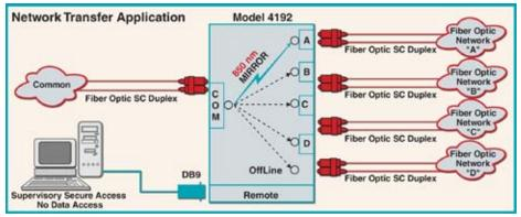
Block Diagram 3: Example of a fiber optic switch with an external Off-Line position.
