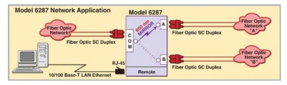
Block Diagram 11: QuickSwitch® 6287 SC Duplex Fiber Optic Mirror A/B Switch with Remote Serial Control via a 10/100 Base-T network.
