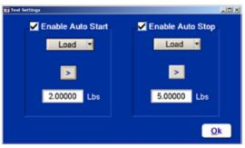
Test Controls - Tests may be automatically started and stopped.
