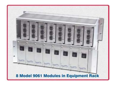
Each Model 9061 module enables access to two 10 Base-T networks. The Model 9061 A/B Switch allows the user to reroute data between two networks with a simple push of a button. The pushbutton face changes color to indicate A or B switch status. The unit supports 4 pins of the RJ45 interface. No need to plug and unplug cables thereby eliminating connector wear.
