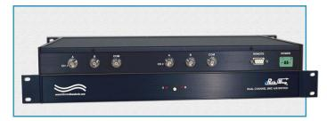
The switch may be controlled locally by manually operating the front panel pushbutton or remotely using the Remote port on the rear. The Remote port allows the user to control switch position using TTL signaling connected to the DB9 Remote port located on the rear of the unit. The front panel LED display indicates the present position and unit power status. Status can also be obtained from Contact Closure pins located on the DB9 Remote port.
