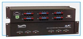
channel is set to Normal or Bypass. Each switch may be controlled manually via a front panel pushbutton or remotely from an RS232 serial port located on the rear of the unit. Switch position status may be attained via the front panel LED display or the Remote RS232 serial port (DB9) located on the rear of the unit. All 8 pins of the RJ48 are switched.
