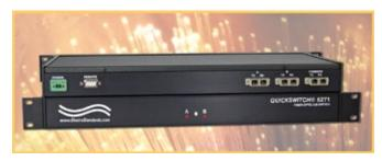
The switch may be controlled locally by manually operating the front panel pushbutton or remotely from the DB9 female serial interface Remote port located on the rear of the unit. The front panel LED display indicates the switch position and unit power status.
