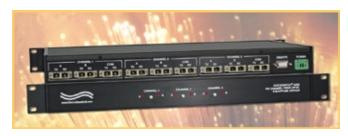
The switch may be controlled manually via the front panel pushbutton or remotely from a DB9 port located on the rear of the unit. Switch position state may be attained via the front panel LED's.
