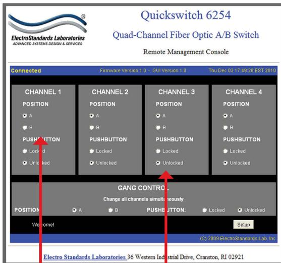
Switch position by selecting "A" or "B" for each channel.
