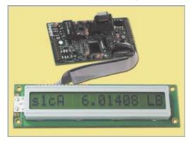
The CellMite® Model 4327 can be fully operated with a computer or simply setup by a computer and then used as a stand alone intelligent digital signal conditioner with auto identifying analog and alphanumeric display outputs.
