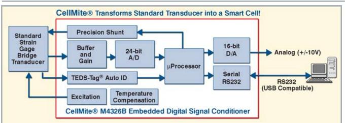
CellMite® is a compact digital signal conditioner unit that can be directly integrated into a standard strain gage transducer such as a load cell or extensometer. CellMite® simultaneously generates a serial digital output for connection to a PC as well as a +/- 10V analog output.
