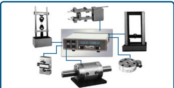
The Model 4215 Smart Indicator connects to a wide variety of tensile testers, extensometers, torque transducers, and other strain gage transducers.
