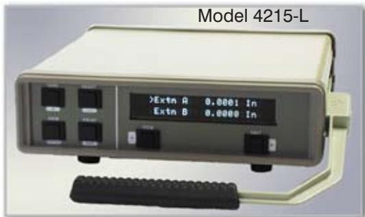
The ESL Model 4215-L Advanced Digital LVDT Meter provides all excitation and signal conditioning necessary to operate dual LVDT expansion measurement fixtures. The average extension is computed automatically and displayed. The ESL Advanced Digital LVDT Meter also features analog outputs, limit switching, individual unit conversion and a two-line display. Factory options support mixing and matching of strain gauge and LVDT sensor inputs.
