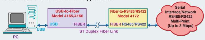
Isolated PC USB to RS485/RS422 communications serial interface/network.
