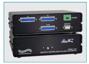
**In Manual A/B Switch Mode**, the Model 4123 may be controlled locally via its front-panel pushbutton, or remotely via its REMOTE control port that accepts RS232 serial data ASCII commands.
